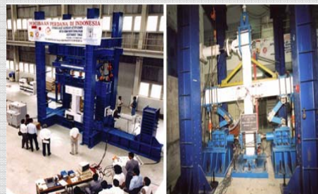
Photo 1. View of an Element Structure Test (White Part: Specimen)
