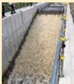
Experiment with large-scale embankment model
