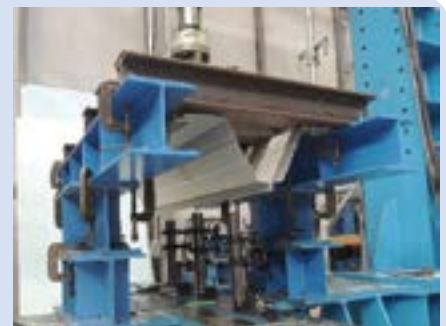
Loading test on joints of folded plate roofs
