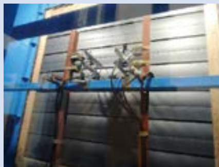
Wind pressure resistance test of metal roofing
