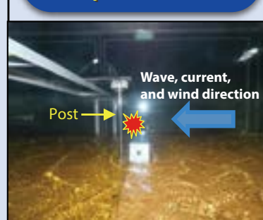
Experiment on impact acting on the posts of drift fences
