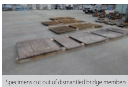
Specimens cut out of dismantled bridge members
