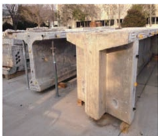
Specimens cut out of dismantled bridge members
