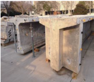
Specimens cut out of dismantled bridge members
