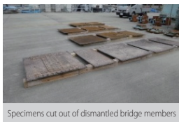
Specimens cut out of dismantled bridge members
