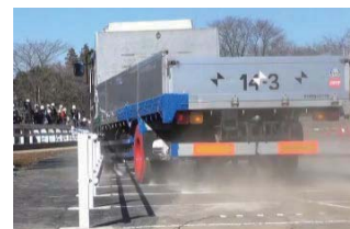
View of full-scale vehicle collision test of guard fences for residential roads
